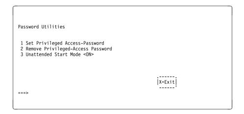
**Set Privileged-Access Password**: The privileged-access password protects against the unauthorized starting of the system programs. When this option is selected, another screen displays that allows the setting of a password.
